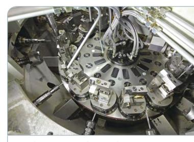
:: Indexing chucks on the Epic R/T machine enable fivesided machining of about 25 different lock body sizes with little to no adjustment from one size to another.
